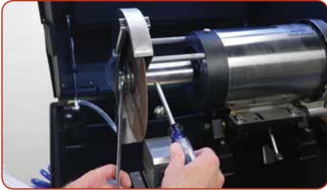
Blades ranging from 8"-10" (203-254 mm) can be easily and quickly changed with provided tools.
