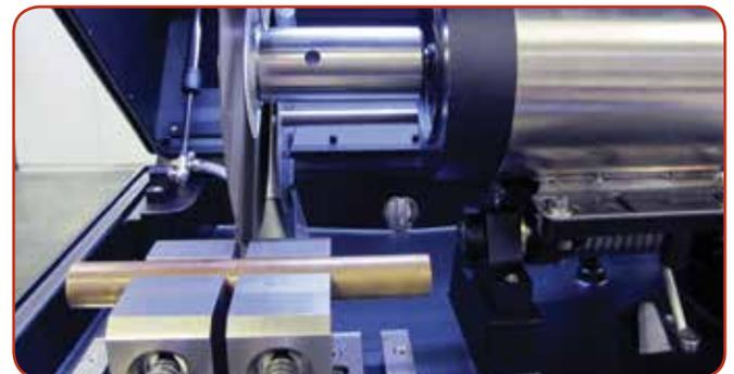
Extra-long 5" (127 mm) distance between the blade and motor allows longer/larger parts to be sectioned.
