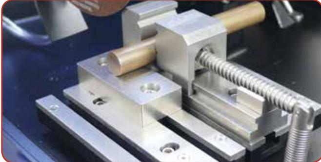
This platform has a height equal to the base of the vise, allowing the unclamped portion of the sample to be supported during the sectioning process. It prevents this portion from falling as the end of the cut nears, minimizing the burr upon completion. It can be positioned anywhere along the T-slots.
