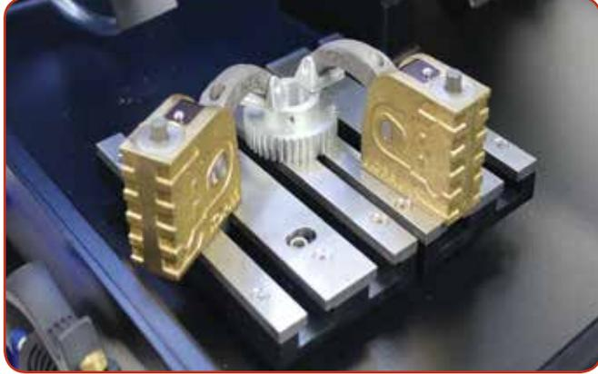
The vertical adjusting clamp can be positioned in any orientation throughout the T-slots in the tables. The height adjustable lever allows various size samples up to 2.25" (57 mm) thick to be secured. Interchangeable pads are available for a variety of sample shapes. Each clamp includes one (1) angled pad and one (1) flat pad.
