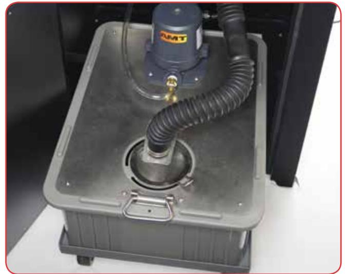
The 7-gallon (26.5 L) recirculating coolant system is constructed of corrosion resistant materials for maximum durability. The reservoir fits conveniently in the available cabinet, or can be placed near the machine in existing lab furniture. A removable catch screen enables quick cleaning of larger particles. Baffles inside the reservoir trap particulates. The optional roller cart (included with cabinet) allows easy transfer for cleaning.
