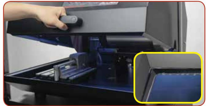
The cover has a large, shatterproof viewing window for operator safety, and an angled internal edge that eliminates external dripping. A safety switch quickly stops blade rotation if the cover is raised during operation.
