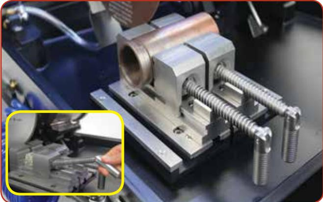
Made of hardened stainless steel, the quick-slide vise features a lead-screw that disengages for quick and easy operation. The vises can be positioned anywhere along the T-slots, and allow samples up to 3" (76 mm) deep to be secured.
